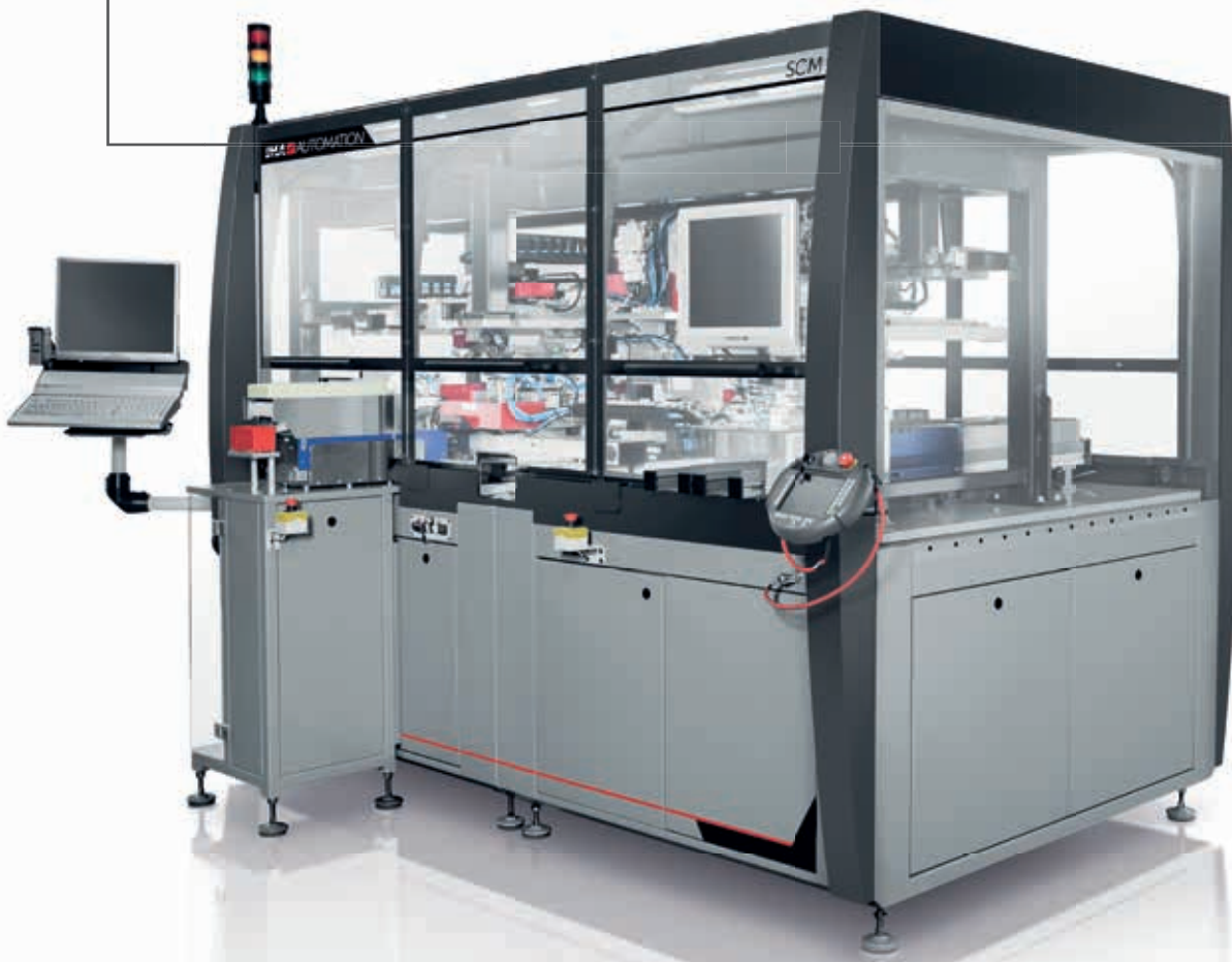
FLEXIBLE LINE FOR CRIMPING AND ASSEMBLING OF SURGICAL SUTURES.
